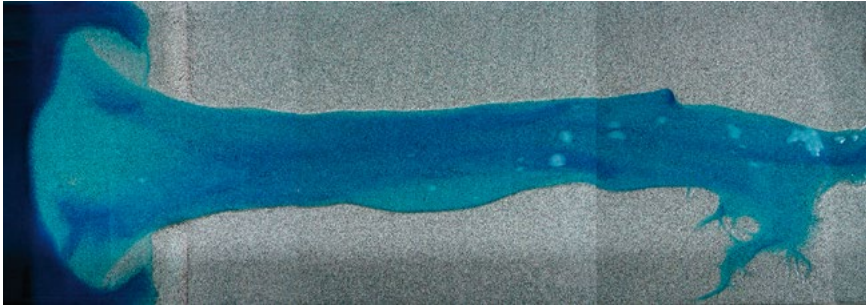
Experimental estuary formed from a straight channel in a periodically tilting flume. Length 3 m (Jasper Leuven). Click on the image to view the full movie.
